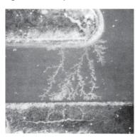
**FIGURE 2.** Shown - Dendrite corrosion between pads on an edge-connector.
